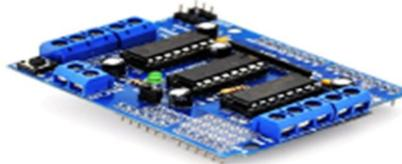
Fig .5 – L293D Motor Driver
