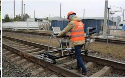
Figure 2. Eddy current testing
