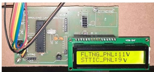
Fig.19 Final output voltage displayed on the LCD
