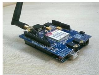
Figure 6. GSM module with Arduino
