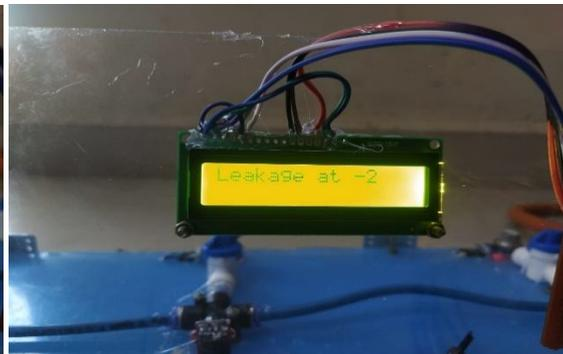
Figure 7. LCD display showing the position of leakage
